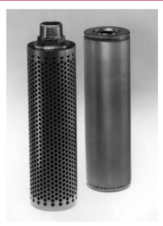
Micro-Screen® filter elements are produced from premium quality woven stainless steel screen mesh. Elements are all-304 or 316 stainless steel, with screen and perforated internal support attached to end caps equipped with replaceable gaskets. Elements can be cleaned chemically or ultrasonically and reused. Cylindrical elements may also be cleaned in place by backflushing. Request literature LITMSPKCLN for recommended cleaning instructions.
